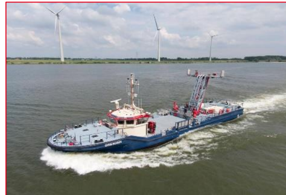
Bedleveler and fire-fighting vessel using a plug-in-hybrid engine
