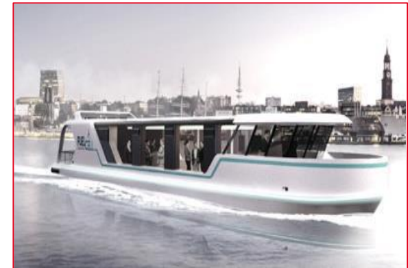
Small passenger ship with methanol fuel cell propulsion
